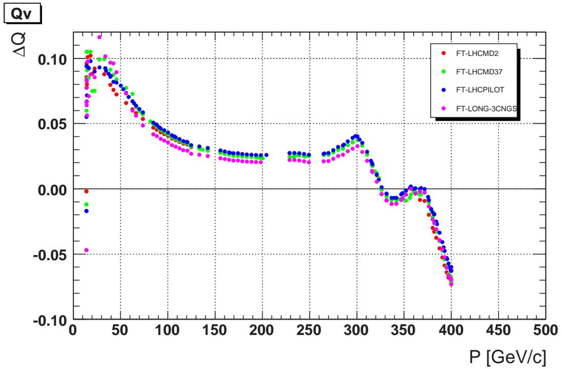
Figure 2: Tune trims for the horizontal (top) and vertical (bottom) plane for FT cycles used in 2007.
