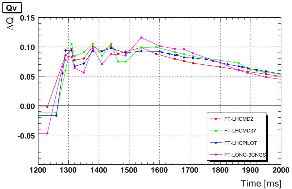
Figure 1: Tune trims as a function of the cycle time in the first part of the FT ramp for the horizontal (top) and vertical (bottom) plane for FT cycles used in 2007. The ramp starts at 1260 ms and the beam crosses transition around 1480 ms.
