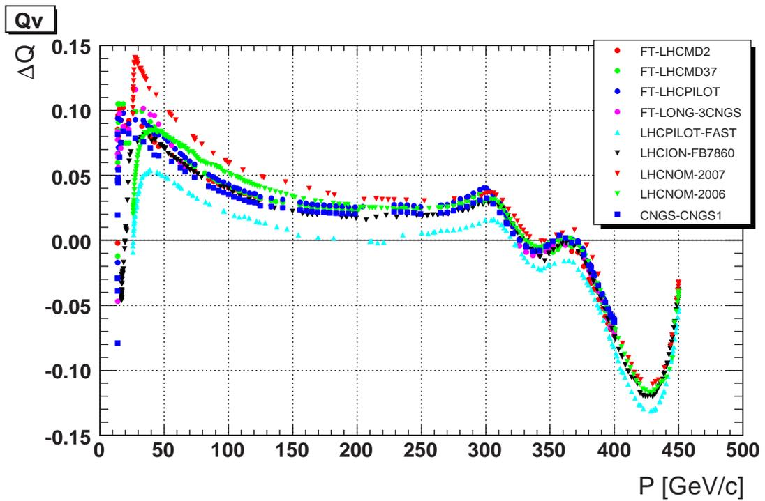
Figure 3: Tune trims for the horizontal (top) and vertical (bottom) plane for a palette of cycles used in 2007 and the nominal LHC cycle of 2006. One notes the difference between the nominal LHC cycle of 2007 and all the other cycles.
