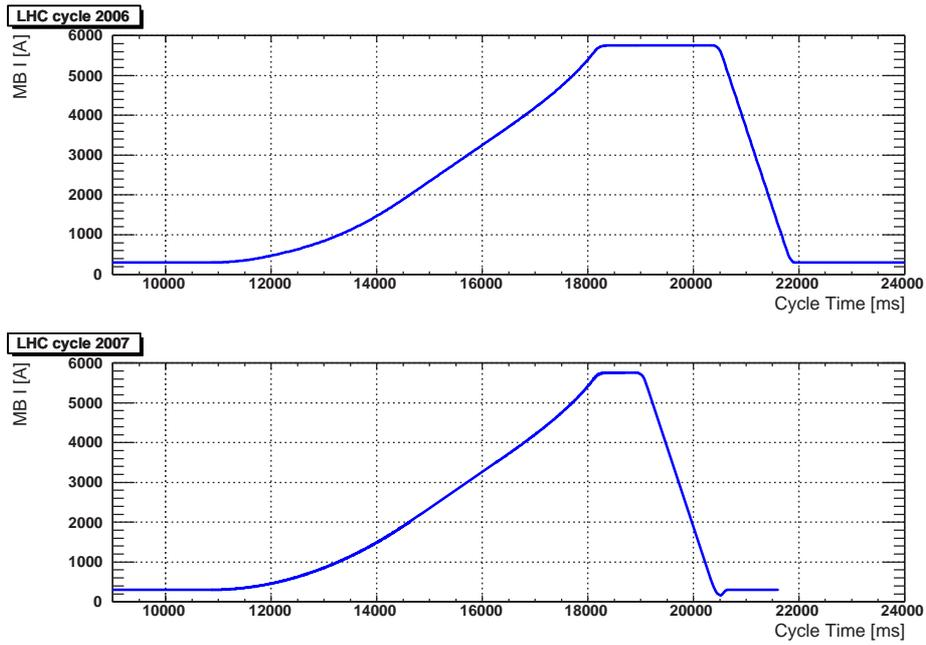
Figure 4: Comparison of the SPS main dipoles current function for the nominal LHC cycle in 2006 (top) and 2007 (bottom). Besides a difference in length of the 450 GeV/c flat top which is not relevant, the significant difference for the tune correction is arising from the small 'degauss dip' to 14 GeV/c (162 A) at the end of the ramp-down.
