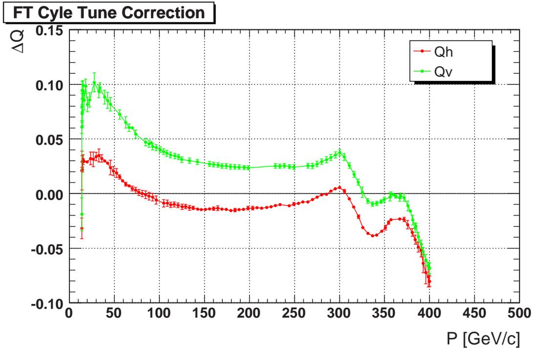
Figure 6: Average tune trims for the horizontal and vertical plane as a function of the beam momentum for the nominal LHC cycle (top) and FT cycle (bottom). For the FT beams the correction corresponds to a total beam intensity of  $\approx 2.8 \times 10^{13}$  protons. For the LHC beams it corresponds to a low intensity beam of less than  $10^{12}$  protons.
