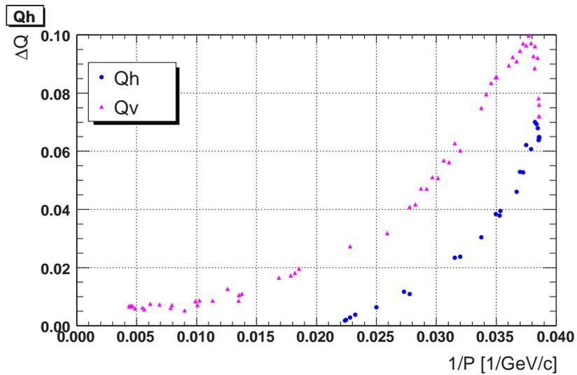
Figure 5: Tune difference  $\Delta Q$  between the tune corrections for the nominal LHC cycle in 2007 and 2006. The difference decays roughly proportionally to the inverse of the momentum in the region of low momenta.
