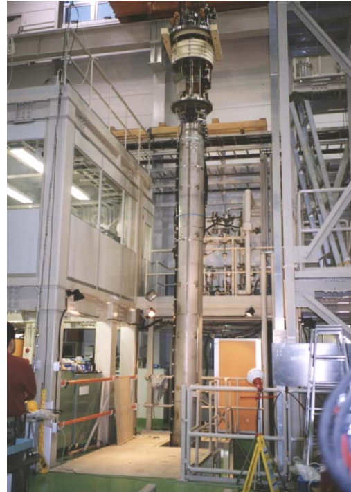
Figure 8.18: (Left) Cross-section of the MQXA low- \beta quadrupole. (Right) MQXA quadrupole ready for tests in the vertical cryostat in KEK.
