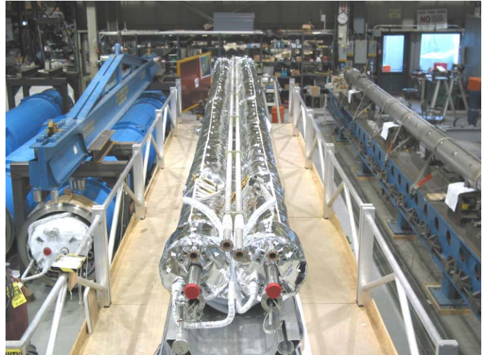
Figure 8.13: (Left) Cross-section of the MBRS dipole. (Right) Assembly of the MBRS cold masses at BNL.
