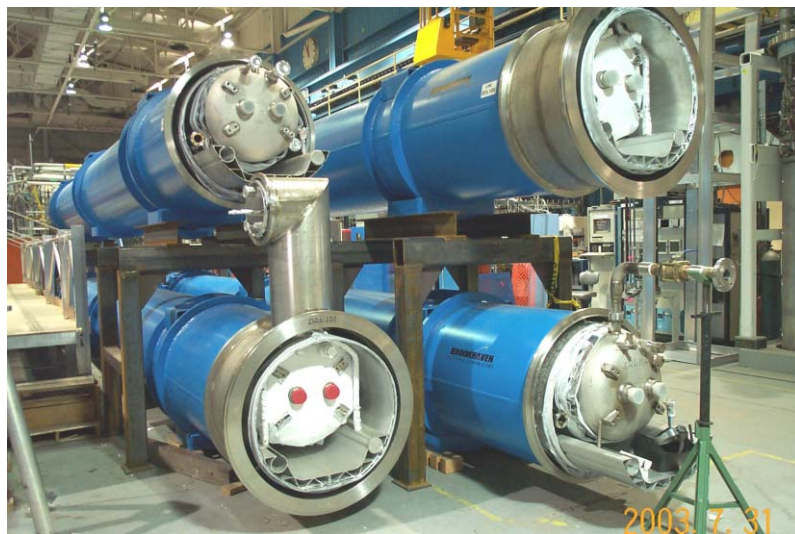
Figure 8.12: MBRB cryo-dipoles ready for shipment. The lower left unit is equipped with a QQS module.
