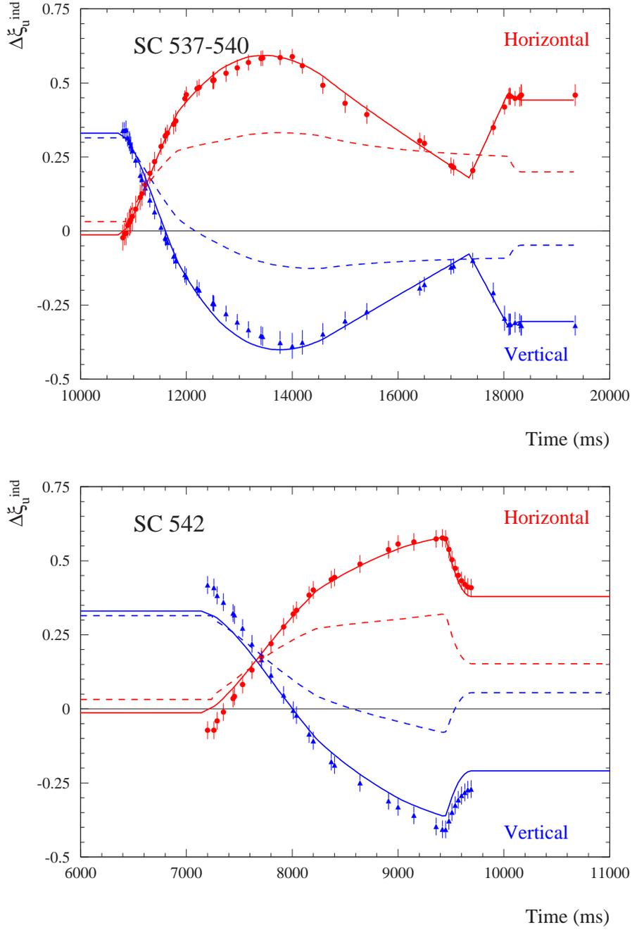
Figure 6: Dependence of  $\Delta\xi_u^{\text{ind}}$  on the time in the cycle for SC 537 and 540 (averaged, top plot) and for SC 542 (bottom plot). Points represent the values reconstructed from the trims and measurements. The dashed line corresponds to the default model with the parameters of column 1 of Table 2. The solid line is the fit to the new model with parameters in column 3 of Table 2.
