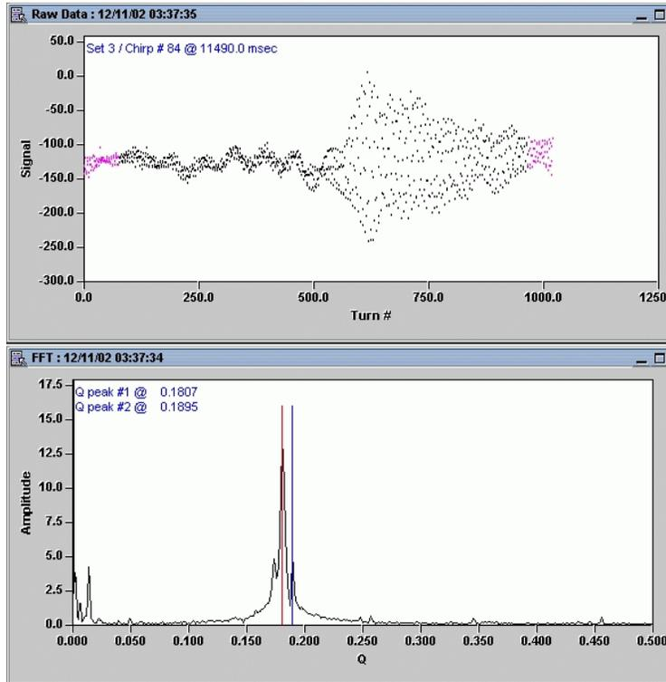
Figure 1: Online MULTIQ raw data display for one chirp sweep : horizontal beam position signal (top) and the corresponding FFT spectrum (bottom). The modulation of the horizontal tune by synchrotron motion is visible on the spectrum. Black dots on the top plots correspond to the duration of the chirp excitation.
