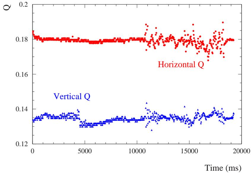
Figure 2: Tune evolution for the SPS super-cycle 540 (LHC beam), recorded with 12 bunches of nominal intensity ( $\sim 10^{11}$  p/bunch) on September 26 2002. Four consecutive MULTIQ measurements are necessary to obtain the full information for each plane.
