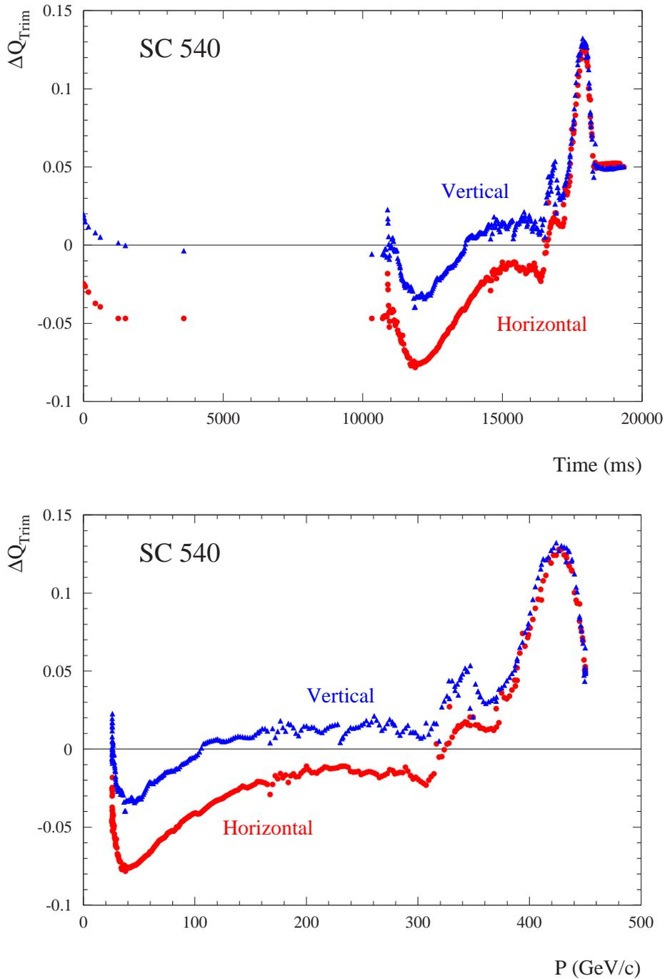
Figure 4: Total tune trim required to obtain the tune functions shown in Figure 2. The trims are relative to the nominal setting for the selected optics and reference tunes. Top : tune trim versus time in the cycle. Bottom : tune trim versus beam momentum. The saturation effects in the magnets starting around 350 GeV/c are clearly visible. The decay of the field in the dipoles at the beginning of the injection plateau is visible from the slowly varying tune trims up to 1000 ms.
