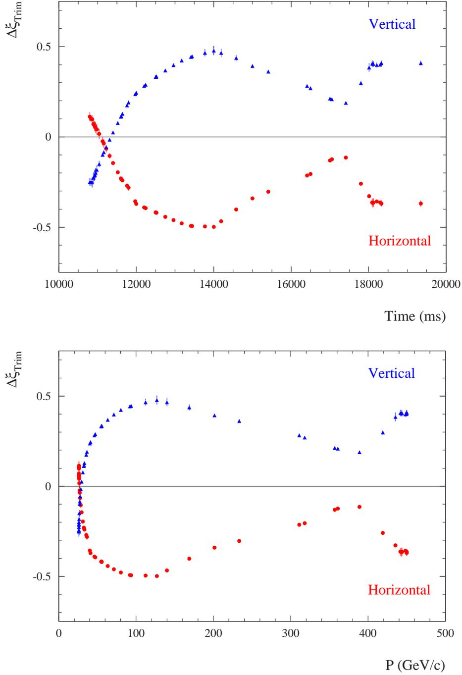
Figure 5: Average chromaticity trims  $\Delta\xi_u^{\text{Trim}}$  applied to the LHC beam cycles (SC 537 and 540) to obtain a chromaticity for the beams of  $\xi_u = 0.075 \pm 0.025$ . The contribution due to  $\xi_u^Q$  is not included  $\Delta\xi_u^{\text{Trim}}$ . Top : chromaticity trims versus time in the cycle. Bottom : chromaticity trims versus beam momentum. Error bars indicate the spread between the two cycles.
