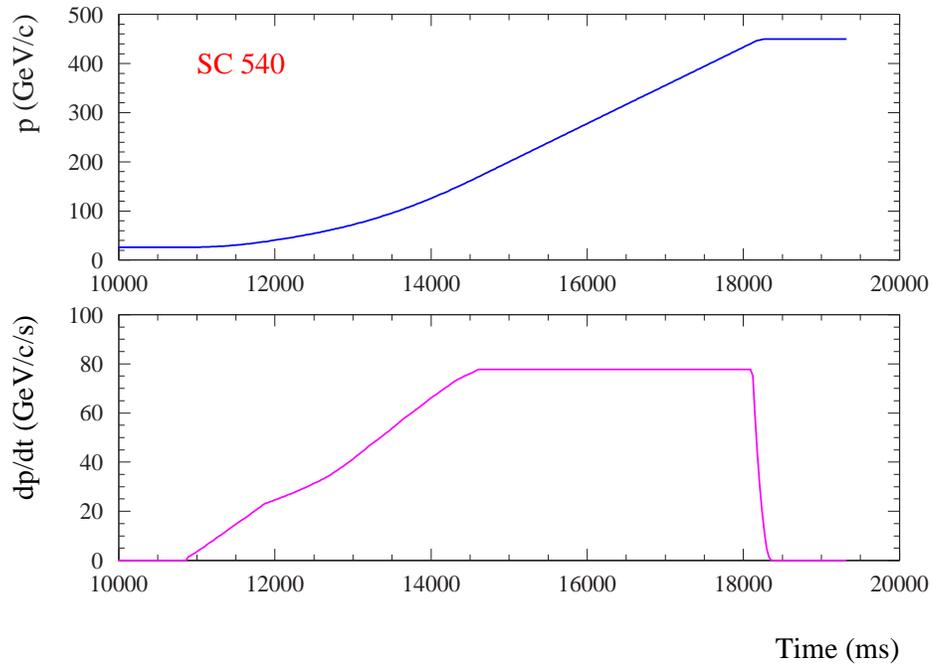
Figure 3: Evolution of the beam momentum (top) and the change of momentum  $\dot{p}$  for the LHC cycle ramp.
