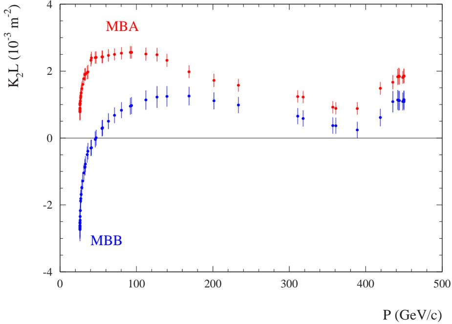
Figure 8: Strength of the sextupolar field components in the main SPS dipoles MBA and MBB as a function of the beam momentum. The data is averaged for SC 537 ad 540 and includes the contributions from eddy currents.
