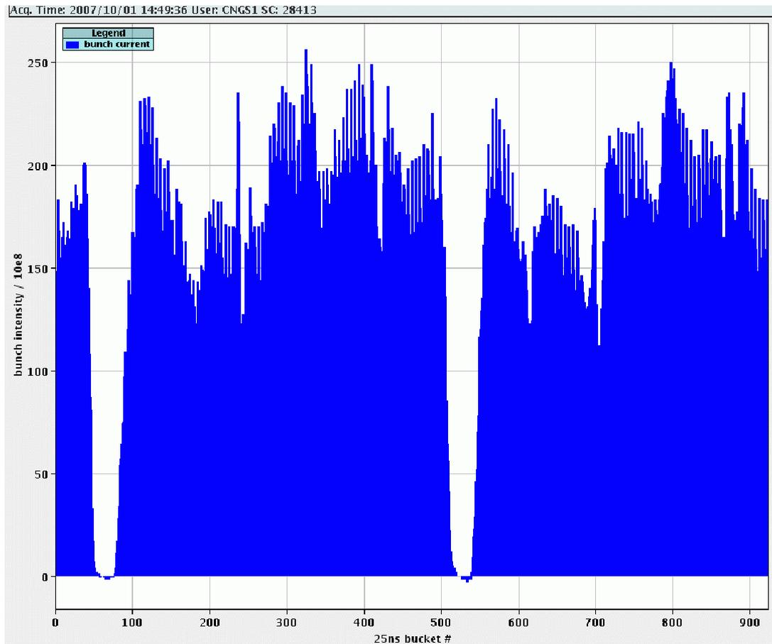
Figure 1: Structure of the CNGS beam with two  $10.5 \mu\text{s}$  batches separated by two  $1 \mu\text{m}$  gaps. Each bin gives the intensity integrated over 25 ns, respectively 5 bunches. The intensity variations within a batch due to the 5 turn extraction from the PS is clearly visible.
