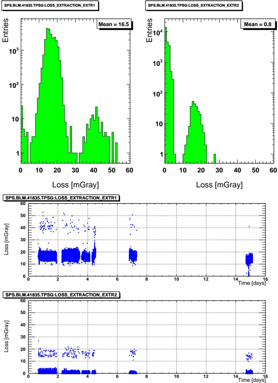
Figure 10: Distribution and time evolution of the measured beam loss on the BLM at the TPSG. A loss of 20 mGray corresponds to  $10^{10}$  protons lost on the TPSG.
