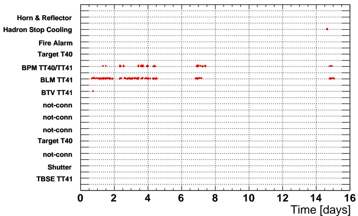
Figure 16: Time distribution of (possible) false interlocks for the two Beam Interlock Controller crates (TT41A and TT41B) that handle interlocks from the TT41 transfer line and the CNGS target and secondary beam area. The vertical scales corresponds to the different input channels.
