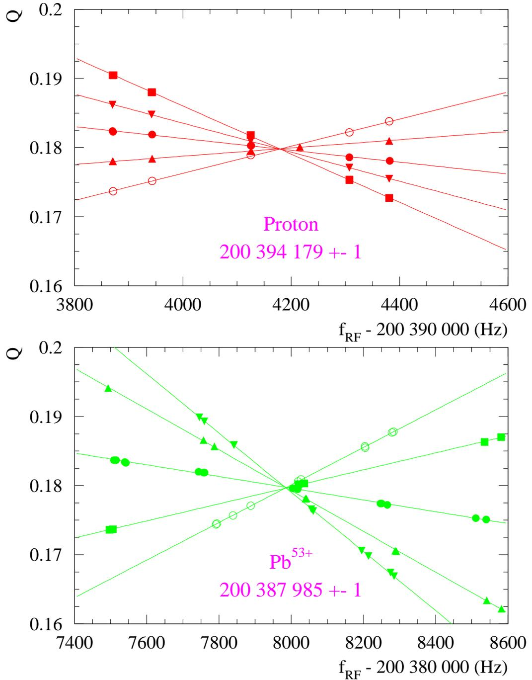
Figure 3: Horizontal tune dependence on RF frequency for different settings of the machine chromaticity for proton (top) and  $\text{Pb}^{53+}$  beams (bottom) at a proton equivalent momentum of 450 GeV/c in the SPS (from Reference [8]). The central RF frequency (and its error) that corresponds to the crossing point is indicated for each beam.
