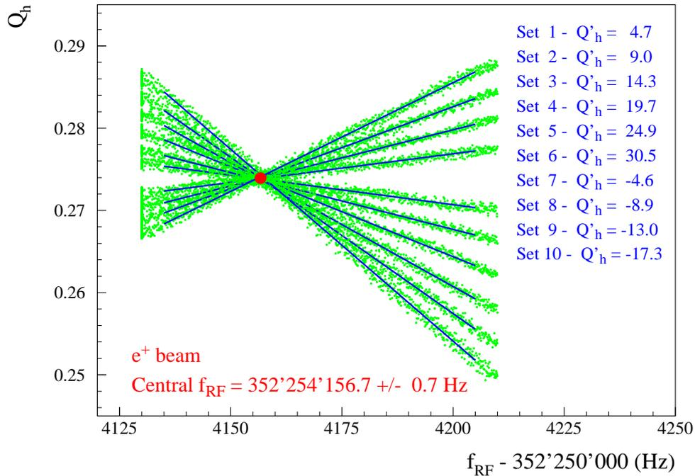
Figure 1: Example of a central frequency measurement at LEP. The tune dependence on RF frequency is measured for a number of chromaticity settings  $Q'_h$ . At the crossing point of the measurements the beam is centered in the sextupoles since the tune is independent of  $Q'_h$ : this frequency setting corresponds to the central frequency. This measurement was based on a PLL (Phase Locked Loop) tune measurement providing data at a few Hz.
