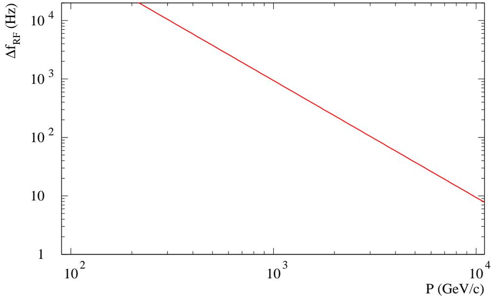
Figure 4: Expected central RF frequency difference between proton and  $\text{Pb}^{82+}$  beams as a function of the beam momentum at the LHC. At 7 TeV/c the frequency difference is only  $\sim 20$  Hz.
