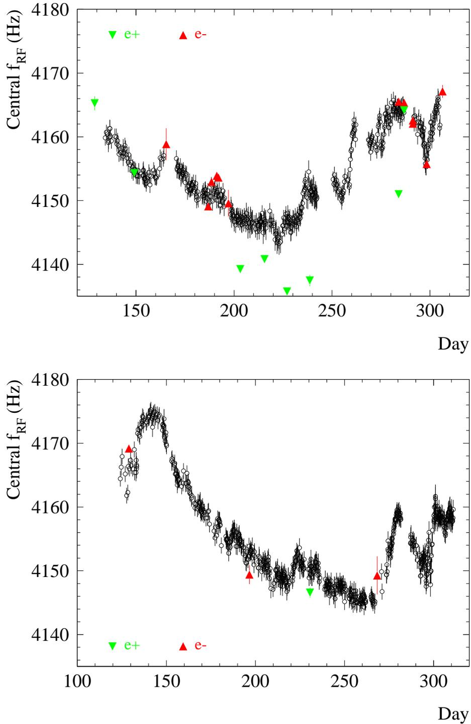
Figure 2: Evolution of the LEP central RF frequency during the 1998 (top) and 1999 (bottom) LEP runs [4]. The open points are obtained from BPM measurements and are normalized to the actual central frequency measurements (filled triangles). Only the last four digits of the central frequency are given,  $f_{RF}^c = 352'25.'\dots$  Hz.  $\Delta f = +1$  Hz corresponds to  $\Delta C = -100 \mu\text{m}$ .
