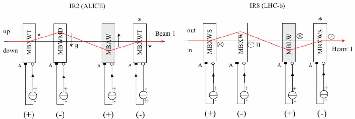
The compensators are powered according to the rules for the orbit correctors in the arc, i.e., a positive kick (upwards or outwards) on Beam 1 is obtained by a positive setting on the bi-polar power supply and the current entering the B terminal of the compensators. Notice the change of polarity for the turned, vertically deflecting magnet MBXWT in IR2 while the turned, horizontally deflecting magnet MBXWS keeps its optical function (see also section 7 on turned magnets).
