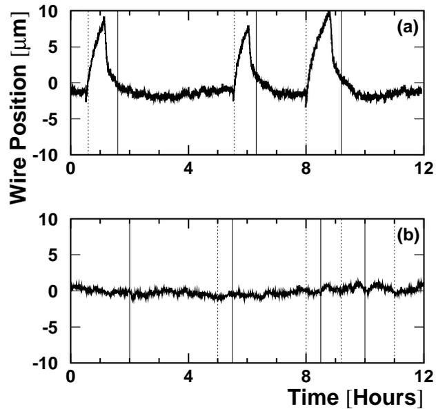
Figure 25: The response of a reference WPS over two 12-hour periods before (a) and after (b) additional radiation shielding was installed, and the wire centred within the sensor. The vertical solid lines indicate the declared start-of-fill and the dotted lines indicate a beam dump. Note that (b) encompasses fills in which actual spectrometer measurements were performed.
